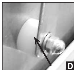
Re-adjust the door springs at the rear of the dishwasher then check that the doors open and close without binding.
